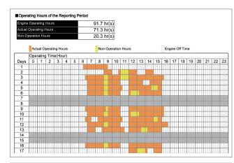
The daily operation report shows in detail when the machine is operating and idle time, which is represented by different colours in the 24-hour timeline.
