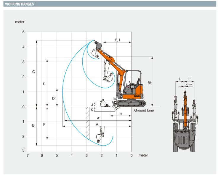
This illustration shows with 1.17 m arm, 0.06 m³ bucket and 300 mm rubber shoes.
