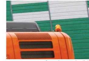
Operation warning lights
