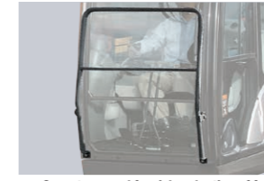
Operator guard for risk reduction of falls
