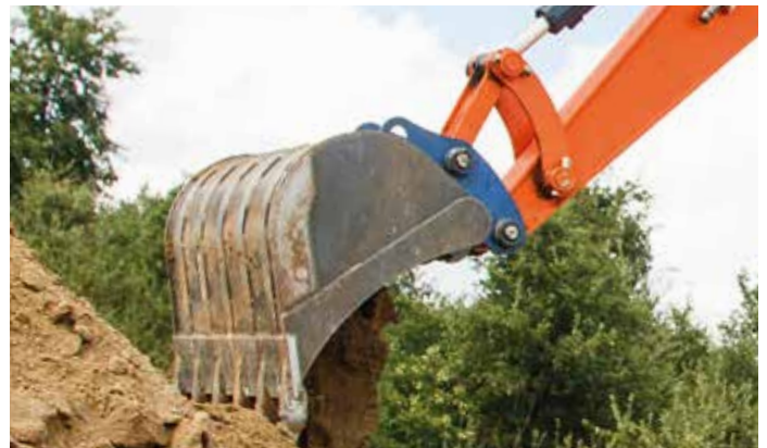
High-quality ground engaging tools include self-sharpening teeth and reliable adapters to ensure a precise fit.
