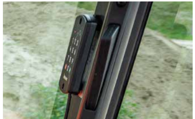
Additional security comes from the control pad immobiliser.
