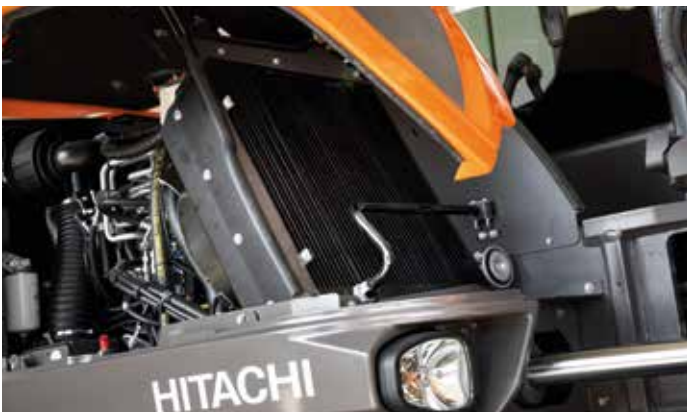
The radiator compartment is easy to clean.
