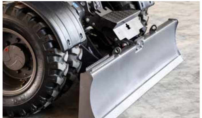
For added convenience and versatility, the blade is prepared for trailer hook installation.
