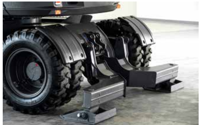
The independently operating outriggers enhance stability.
