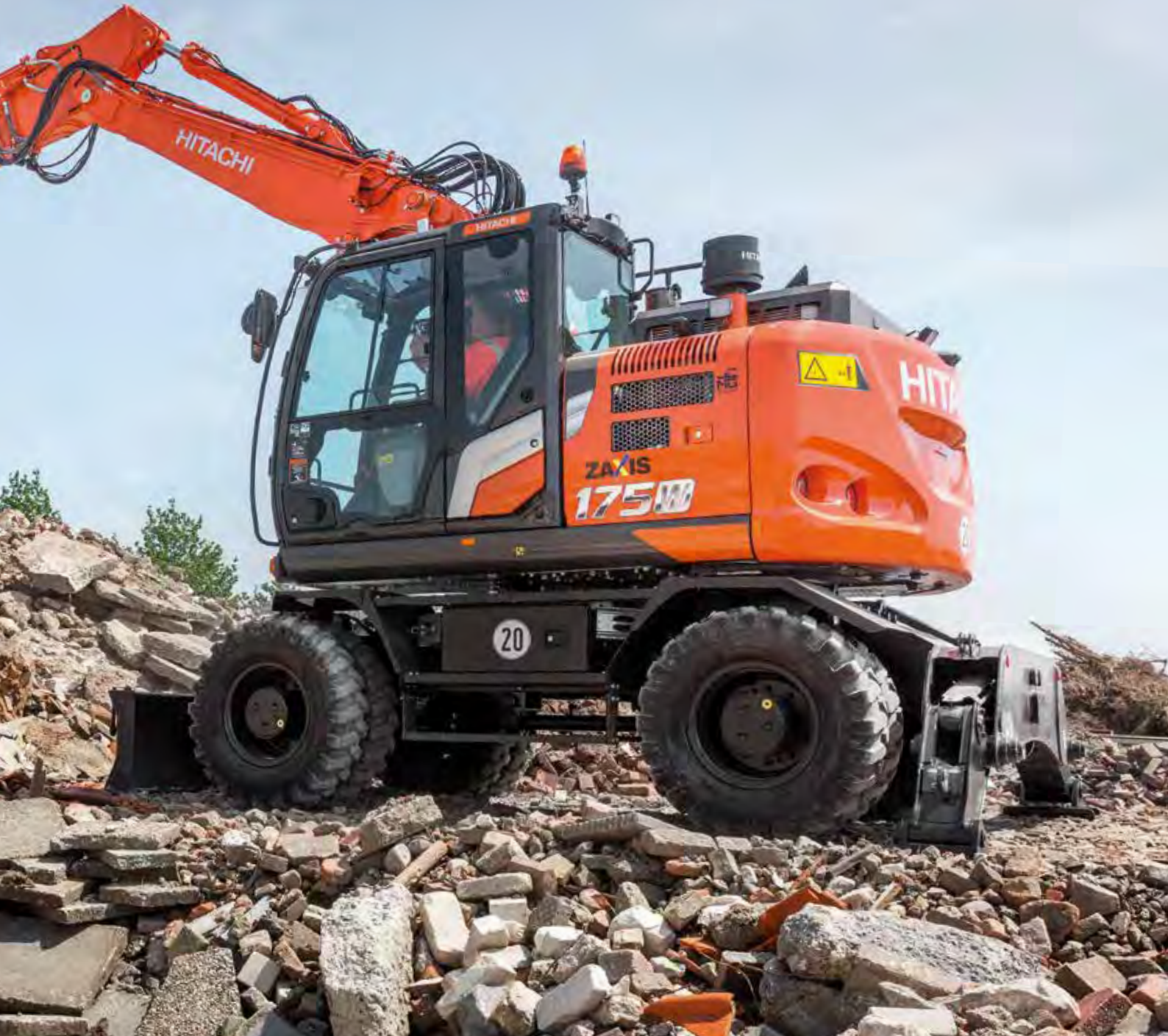
HIOS V hydraulic system increases front speed and reduces fuel consumption.
