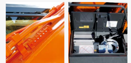
Centralized boom and arm greasing points Electric grease gun with hose-reel (Optional)
