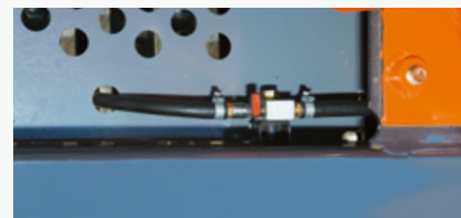
Fuel tank water drainage cock
