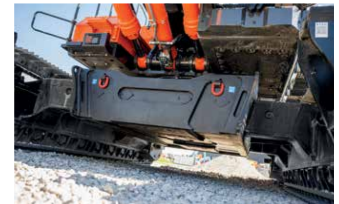
The undercarriage of the ZX400MC-7 and ZX600MC-7 extends for stability.
