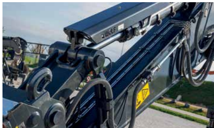
The ZX390TC-7 has bucket cylinder protection to enhance durability.
