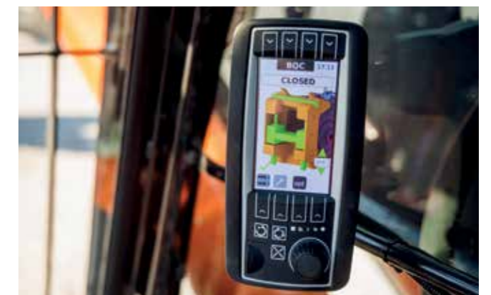
The boom can be changed quickly from the cab using Boom Quick Connect technology.
