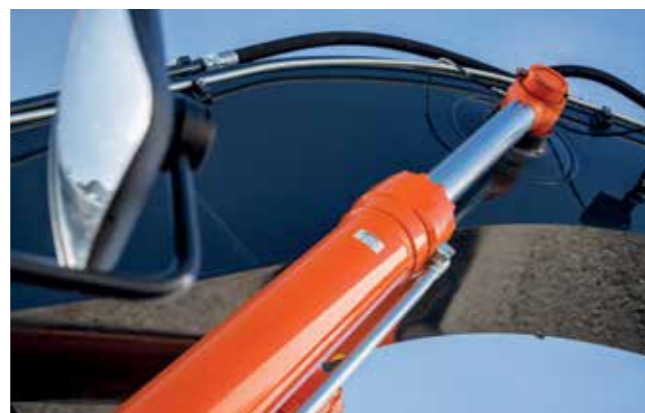
Larger boom and bucket cylinders on the ZX390TC-7 enable it to work with heavier tools.
