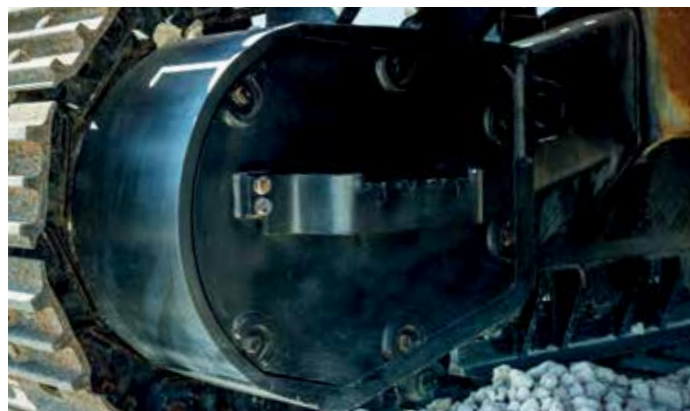
Reinforced travel drive covers offer protection in tough working environments.
