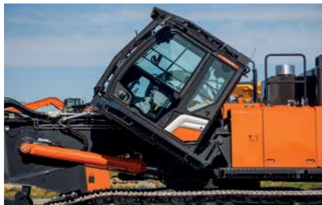
Tilting cab of the ZX400MC-7 and ZX600MC-7 gives excellent visibility.
