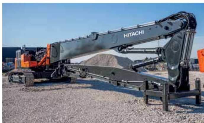
Easy-to-use stands for storing front equipment on the job site and transport.
