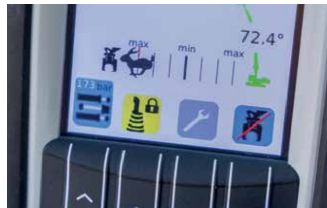
An alarm indicates if the permitted working range is exceeded (the tool speed is then automatically reduced).
