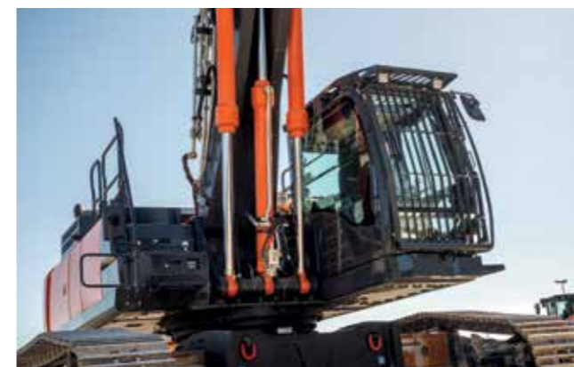
The triple boom cylinder enhances the versatility of the ZX400MC-7 and ZX600MC-7.
