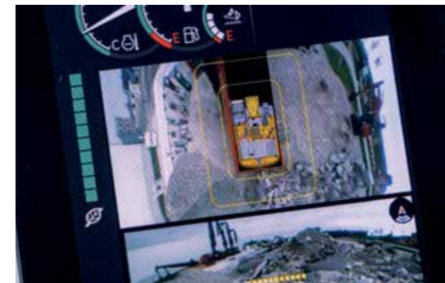
Camera systems give the operator multiple views of the job site.
