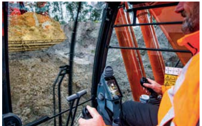
Wider wiper design provides greater visibility.
