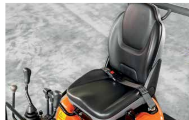
Sliding seat with relocated seatbelt, engine cover handles and reclining stopper.
