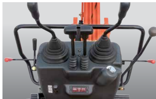
The ignition switch is easy to access and the monitor shows status indicators at a glance.
