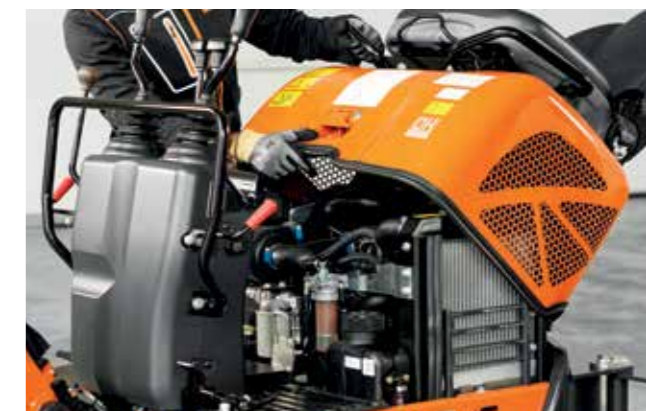
Wide-opening covers allow for easy maintenance.
