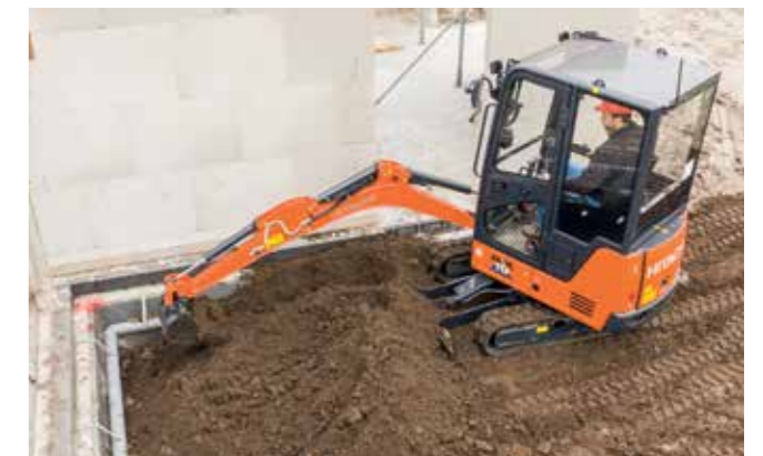
Small front minimum turning radius is ideal for narrow spaces.
