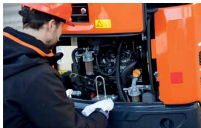
Daily inspection points are grouped together for convenience.
