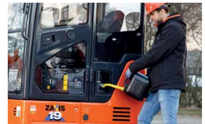
Relocated fuel tank opening allows for easy refuelling.
