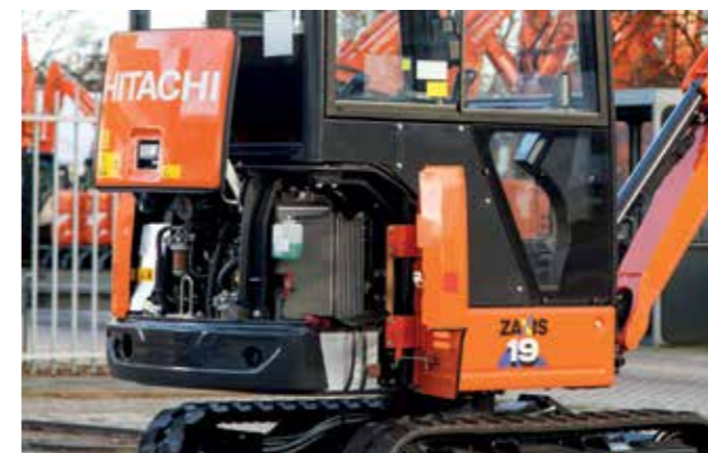
The engine cover opens vertically, which is ideal for tight spaces.
