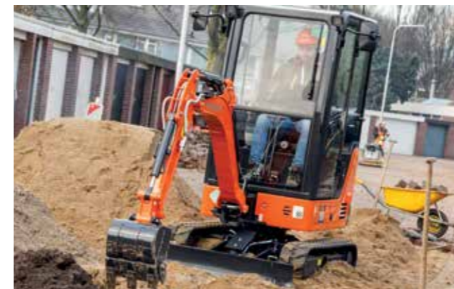
Hydraulic hose on the front attachment is inside the boom for added protection.
