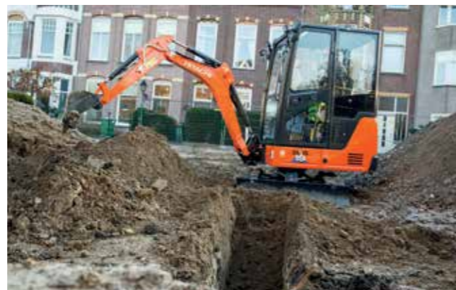
The boom cylinder on top of the boom minimises downtime due to reduced contact with the cylinder.
