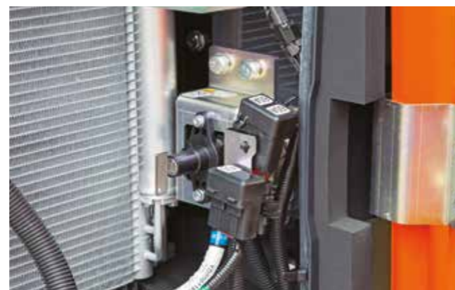
The battery disconnect switch allows maintenance to be carried out safely.
