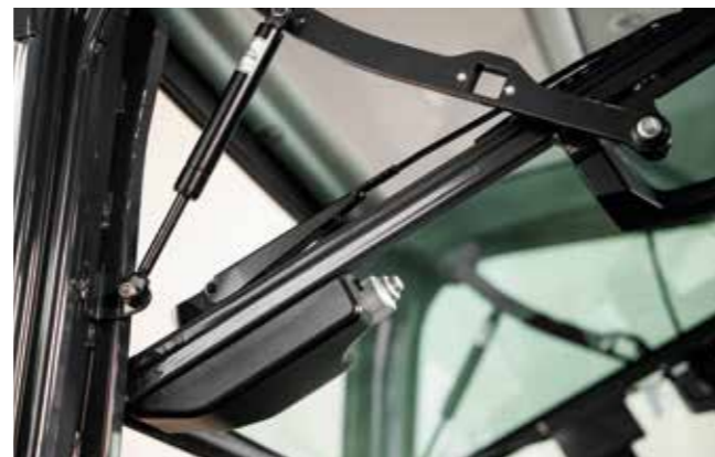
Front window opens smoothly and easily with power-assist function.
