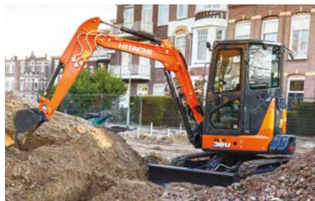
The short-tail swing radius makes the ZX38U-6 ideal for working in tight spaces.
