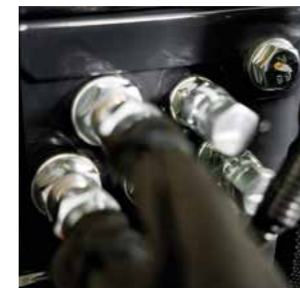
Quick coupler port connection (optional) under toolbox allows for secure retrofit installation.
