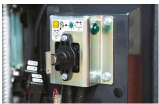
The battery disconnect switch allows maintenance to be carried out safely.
