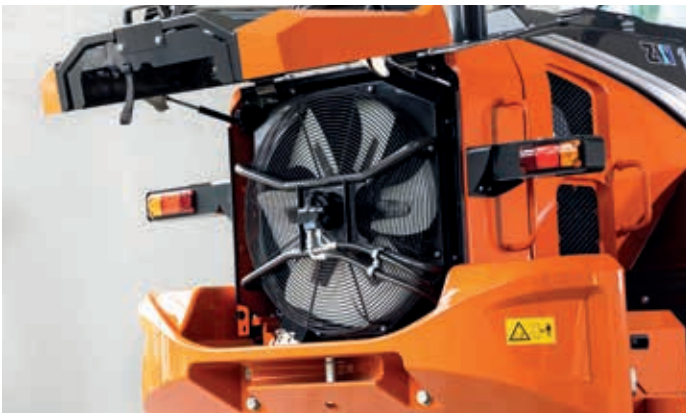
Intelligent fan operation system prevents radiators clogging.
