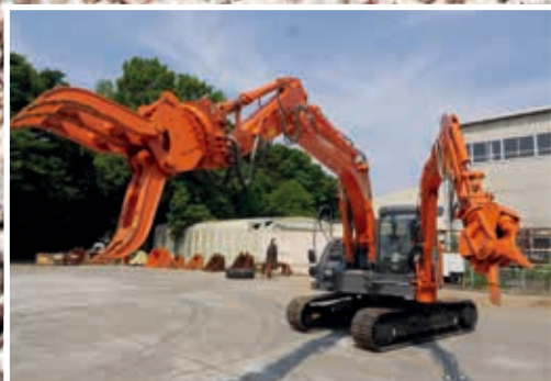
ASTACO (Advanced System with Twin Arm for Complex Operation)
