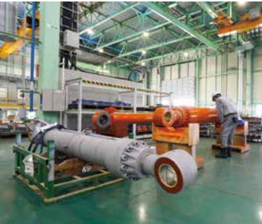
Remanufacturing process of used cylinders at the Hitachinaka Works factory.
