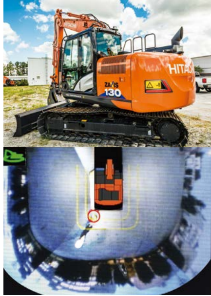
"Aerial Angle" allows operator to check the bird's-eye view image centered on the machine on the monitor in the cab. It improves driving safety and contributes to reducing contact accidents.
