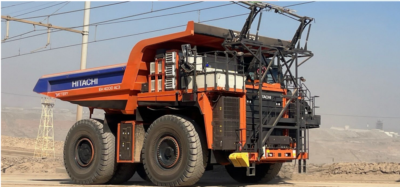
A full battery rigid dump truck based on the EH4000AC-3
