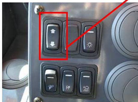
Screen Changeover Switch.
