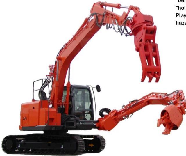
The operation system that enables the simultaneous operation of both arms
