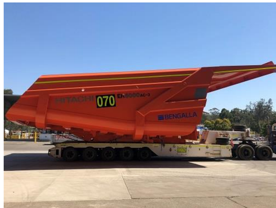
Dump body manufactured at Bradken's Ipswich factory, in Australia. Weight reduced by 10%. (Delivery started in September 2019.)
