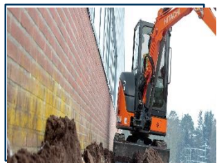
Short swing design for narrow spaces
