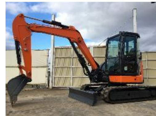
Battery-driven 5t class short swing design prototype
