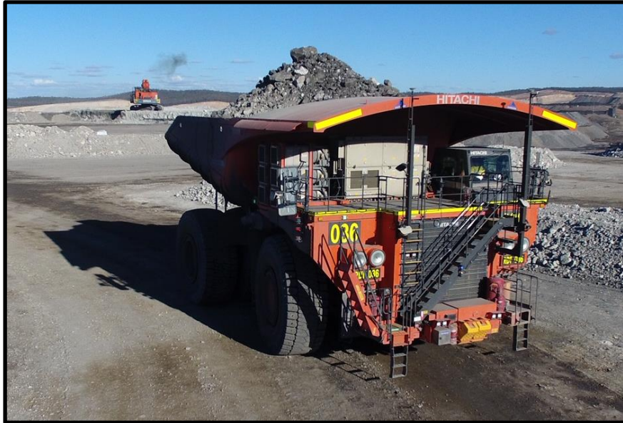
The dump truck EH5000AC-3 equipped with AHS
