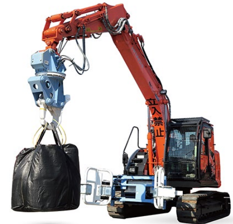
Small sized mobile crane specification machine for radioactive waste sandbags
