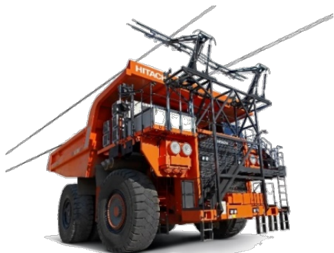
Rigid Dump Truck with Trolley developed in collaboration with Hitachi Group
