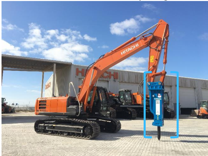
Reference photo: The Hitachi Construction Machinery Middle East hydraulic excavator, to which a breaker is attached, from the same manufacturer as the donated breaker
