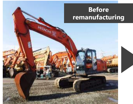
ZX200-3 that was remanufactured at the Hitachi Naka Works (Sold in 2007, suffered water immersion in heavy rain)
