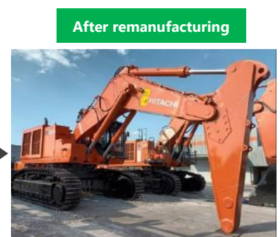
Ultra-large hydraulic excavator that was remanufactured in Zambia (Sold in 2011, 21,950 operating hours)
