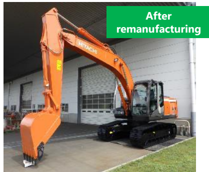
ZX200-3 that was remanufactured at the Hitachi Naka Works (Sold in 2007, suffered water immersion in heavy rain)
