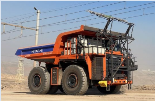
Technological Feasibility Trial of an Ultra-Large Full Battery Dump Truck at the Kansanshi Copper Mine
