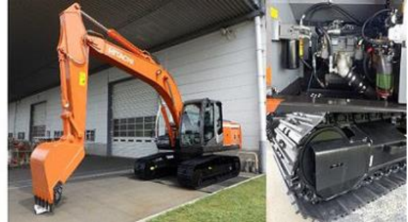
Comparison of before and after remanufacturing of the excavator
