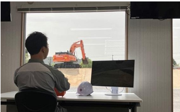
The remote operation of a base machine of hydraulic excavator
