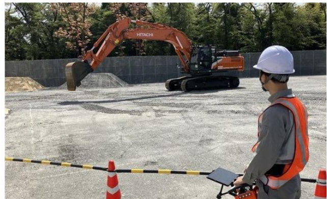
The remote operation of a base machine of hydraulic excavator
