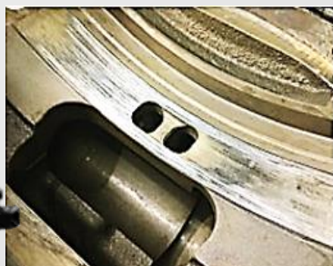
The actual picture of Inner parts of a damaged (scratch) main pump
