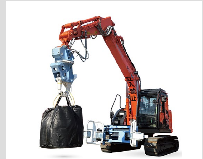
Small sized mobile crane specification machine for radioactive waste sandbags
