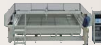
"FS Line", an ultrasonic inspection system for large glass substrates used in flat panel displays
