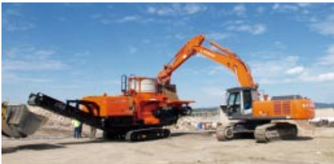
SR2000G track-mounted soil recycler (left) at work in Australia
