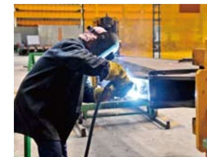
Welding of arm for hydraulic excavator
