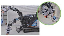
ASTACO-SoRa can handle a wide range of tasks by switching the tools attached to the end of its arms. The remote control has a numerous functions that assist the operator and offers a high level of operability.
