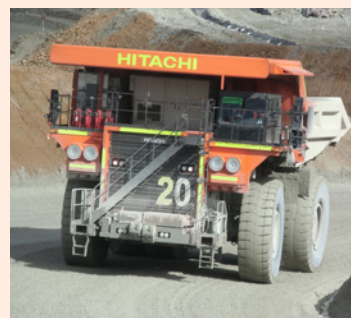
The EH4000AC-3 high altitude dump truck during real world testing
