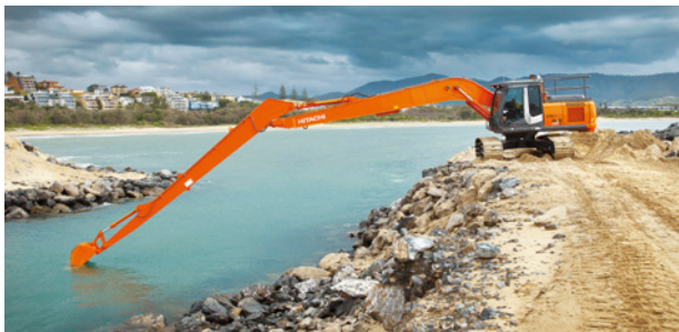
The model with extended reach makes river dredging work even more efficient. Pictured is the ZX240LC (18-meter front) operated in Australia.
