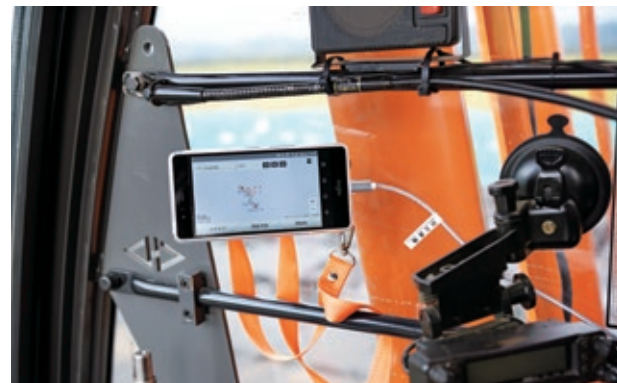
Solution Linkage Mobile's map screen. The location information and list of machines and workers with GPS receivers is displayed using icons.
