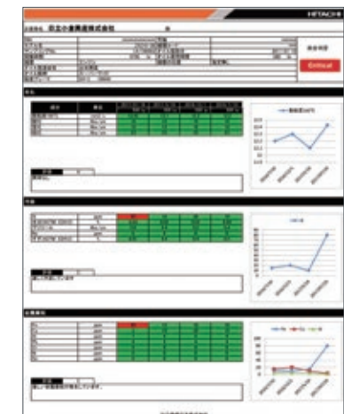
ConSite OIL analysis report prepared automatically. Combining these with operating status reports from ConSite reveals details of machine usage.
