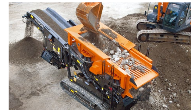
Track Mounted screen can be used to sort and process earth and soil at the scene of a disaster.
