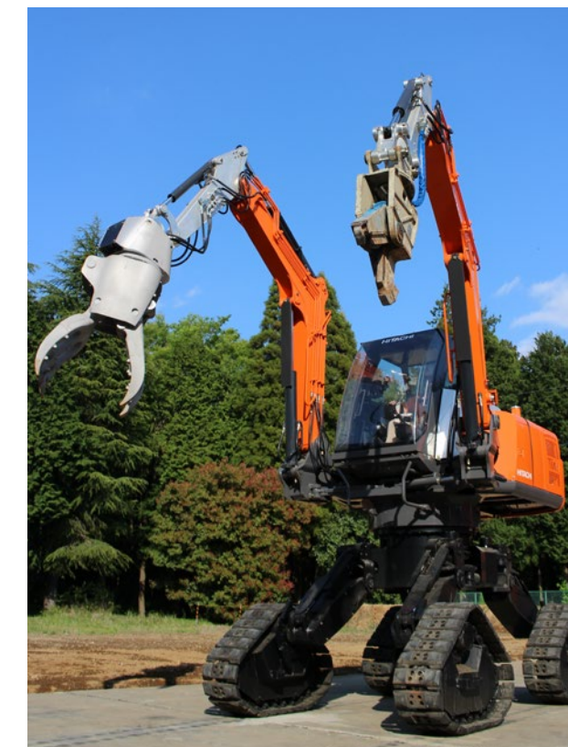
Double-Arm Working Concept Machine with Four-Crawler
