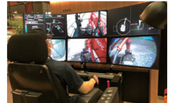
An operator remotely controls an excavator while watching images projected on monitors.
