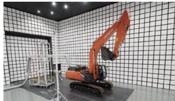
EMC testing of a hydraulic excavator (30-ton class) (image)
