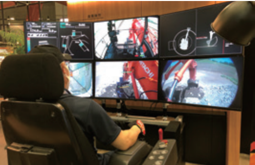
An operator remotely controls an excavator while watching images projected on monitors.
