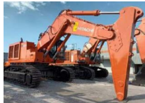
Ultra-large hydraulic excavator that was remanufactured in Zambia (Sold in 2011, 21,950 operating hours)
