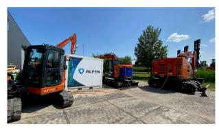
Hitachi Construction Machinery's battery-driven excavators powered by Alfen's mobile storage system
