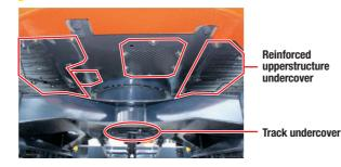
The upperstructure bottom provided with a reinforced upperstructure undercover. And a track frame bottom provided with an undercover. The hydraulic equipment housed inside is protected from rugged ground with rocks, etc.
