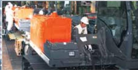
Mid-sized excavator assembly line
