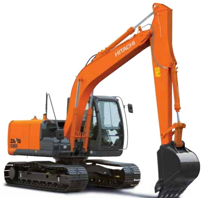
Note: The photos in this brochure show excavators equipped with 3.01 m reinforced arm, 0.45 m³ bucket.
