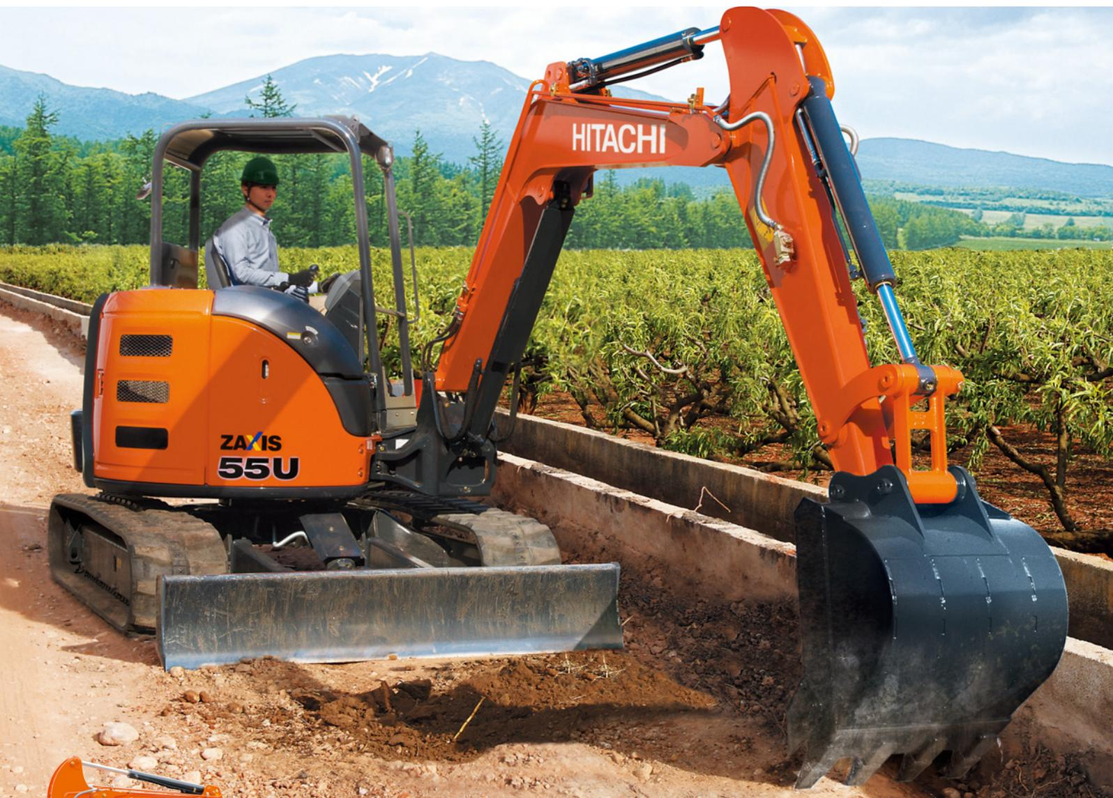
Shown equipped with 1.69 m arm, additional counterweight, armrests, extra piping and pedal as optional items.
