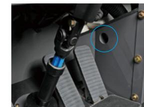
A new vent positioned for the lower legs.
