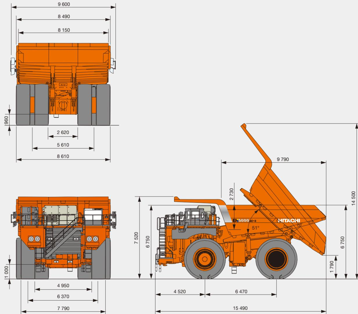
Note: Dimensions shown are for an empty machine with 53/80R63 tires.
