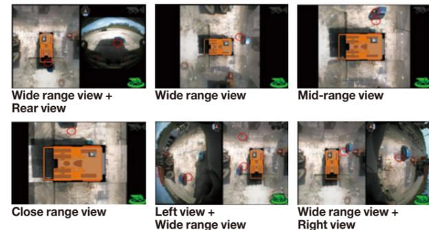
Obstacle Detection (When Stationary) - Supports safer checks before operating
