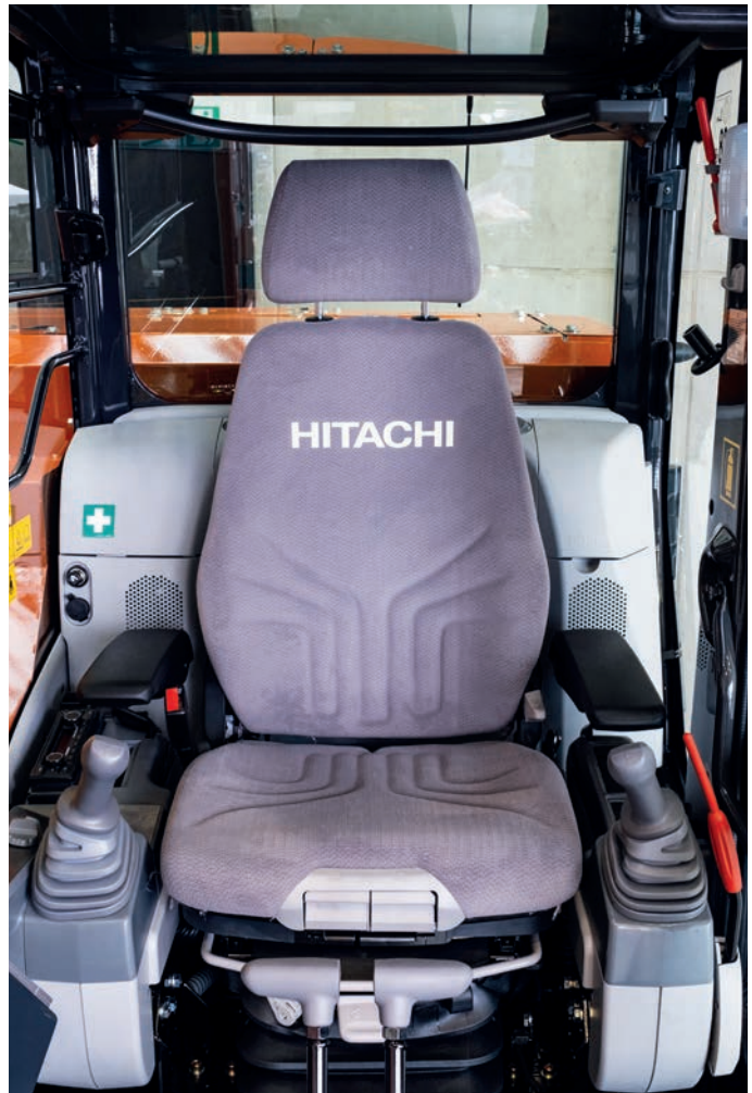
The Grammer comfort seat with seat heating and air springs can be moved for extra leg room.
