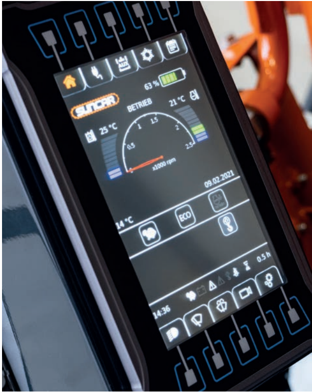
The multifunction monitor is actuated via the ergonomically positioned smart control (rotary-push button).
